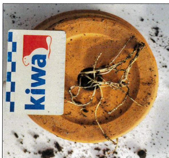
Reference sample at the end of test (roots penetrated bitumen layer and grew through complete pot)
