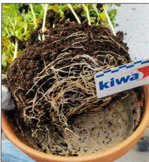
exemplary test specimen at the end of test (no root penetrations)
